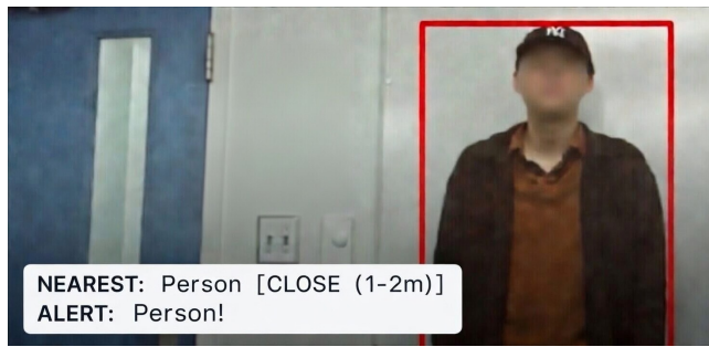
Figure 4: EchoVision output: YOLO detection with SAM segmentation mask and proximity classification.
